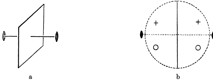
Fig. 35a and b. Symmetry elements (a) and stereographic projection (b) of the class 2/m
