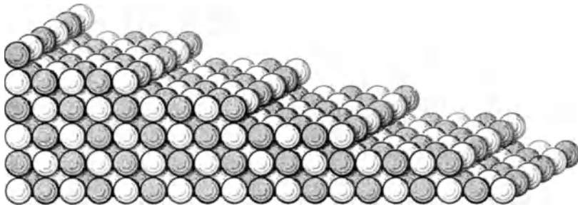
Fig. 277. Model of vicinal plane formed from widely spaced steps; and with very small angle of inclination
