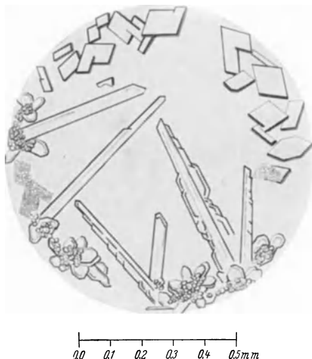
Fig. 290. \text{KNO}_3 crystallization by evaporation under the microscope. The first-formed rhombohedral crystals are transformed upon contact with the later forming orthorhombic needles (middle right). In their vicinity the rhombohedra are dissolved (left above)
