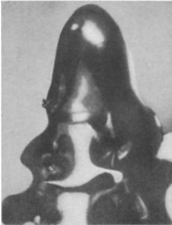
Fig. 279. Point of a copper dendrite ( \times 350 ). (After GRAF)
