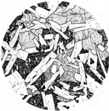
Fig. 314. Pyroxene andesite (Sababurg, Reinhardtswald, north of Kassel). Plagioclase (white) partly lath-shaped in orthorhombic pyroxene (gray with fractures), both in fine-grained groundmass
