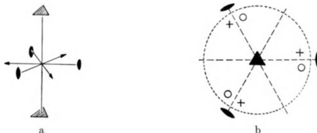
Fig. 55a and b. Symmetry elements (a) and stereographic projection (b) of the trigonal trapezohedral class 32
