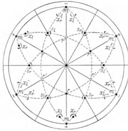
Fig. 59. Stereographic projection of the common faces of quartz. ● positive, ○ negative, ↷ right, ↶ left forms
