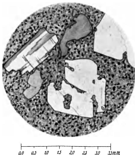
Fig. 295. Rhyolite, Colmitz, Saxony; between crossed nicols. Large corroded quartz and a feldspar with twin lamellae in a fine-grained groundmass of quartz, feldspar and mica
