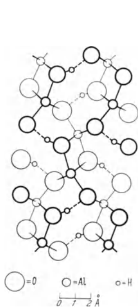
Fig. 167. Atomic arrangement in diaspore. The light and dark circles are actually located in separate planes; the distance between these planes is 1.42 \text{ \AA}
