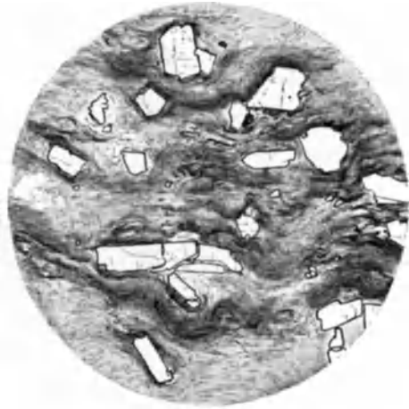
Fig. 315. Flow texture in rhyolite (Grantola by Luino, Lake Maggiore). Phenocrysts of sanidine in a glassy groundmass
